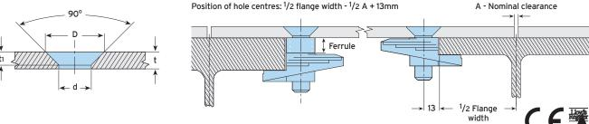
Material: Malleable iron, zinc plated or hot dip galvanised. Stainless steel grade 316.
